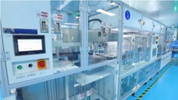
Polarizer & glass bonding line
